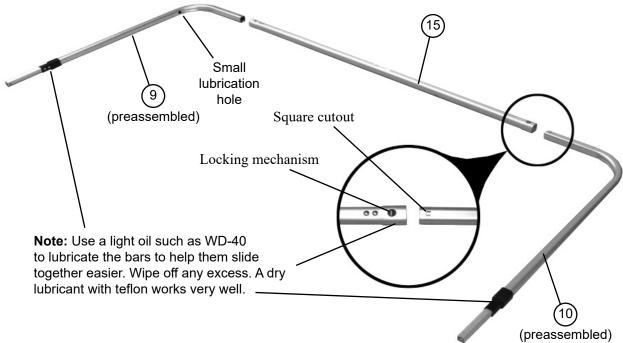
Note: These two assemblies are for the Back and Center Main Frame Bars.
