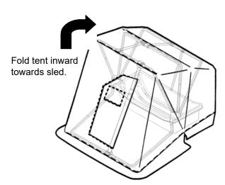
General Note: Be careful with tent windows in cold weather, as creasing or crushing them will cause breakage.
