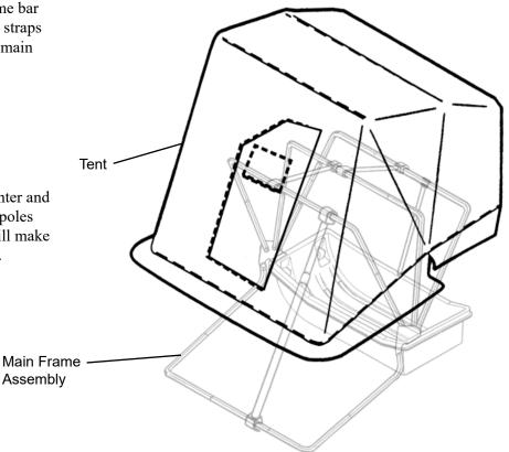
23. Once the canvas is on the frame and the Velcro attached, extend all of the frame bars upward and make sure all of the support poles are installed. Extend the front adjustable support pole so that the fabric in front is snug and not sagging. It will be necessary to loosen the back adjustable pole to achieve this. Once the front is set and the top support poles are in place, the back adjustable pole can be extended until it is snug. Install the plastic trim lock in the positions shown below.
