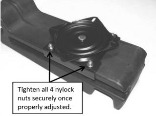
3. Line up the swivel with the inserts in the bottom of the seat. Loosely install the 1/4" x 3/4" phillips head bolt with washers (included in the seat box) into the inserts in the bottom of the seat. Tighten all 4 bolts securely once the swivel is properly positioned.
